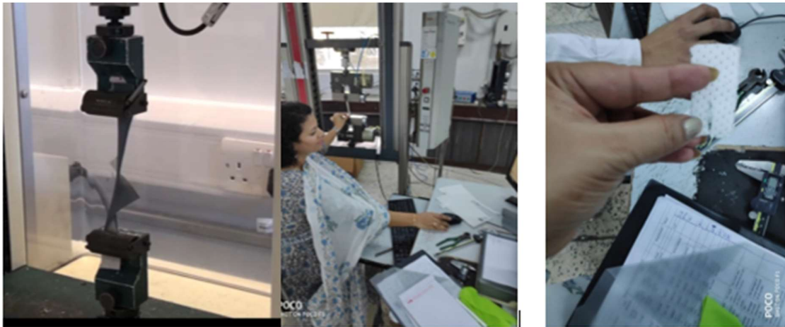
Fig:3.3.3 shows mechanical operation during the tear strength test.
