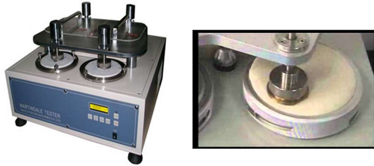
Fig 3.3.4 Martindale tester machine used in testing abrasion resistance.
