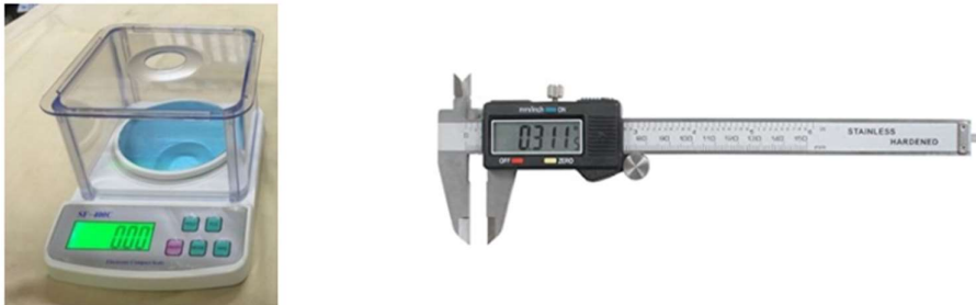
Fig 3.3.1 Instruments used in measuring weight and thickness of Fabrics used in the construction of shoe orthotics.
